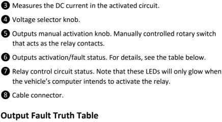
Only one of the two outputs 87 or 87a can be activated at the same time! Fault LEDs on each channel (87 and 87a) will light up when NO load is connected to the corresponding output and the output is not activated. NO load means that the output is left open. Also, the fault LED(s) will light up if any of following fault conditions occurs: Short circuit to positive supply (KL30; +12V; +24V), short circuit to GND or overload. For details, see the table below.
